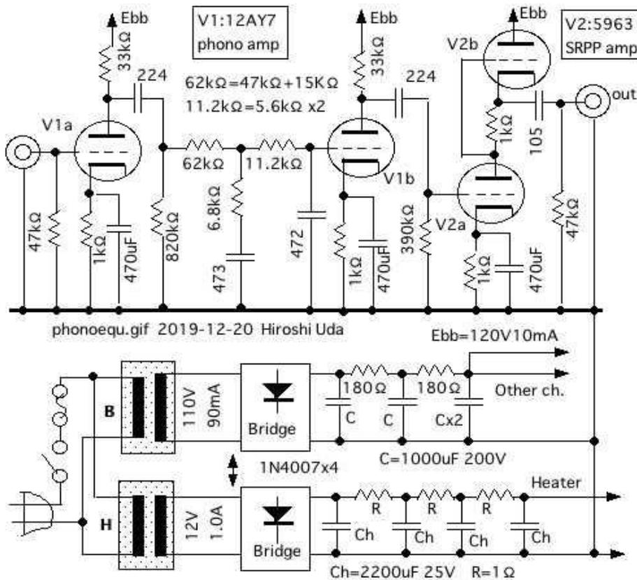
Fig: Schematic of RIAA phono equalizer
